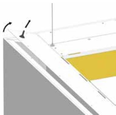
Turn the lamp a quarter (1). Push it to the front, until it comes out of the holder. (2). Pull the lamp to the top.(3)
